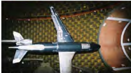
Turbo Powered fan Simulator (TPS) In Rear Fuselage Nacelle configuration
