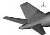
Turbo Powered fan Simulator (TPS) In Rear Fuselage Nacelle configuration
